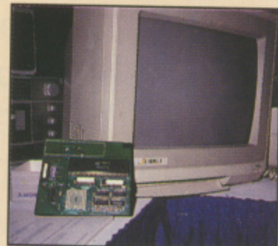
The 14Mhz upgrade from CMI - A1000 model
